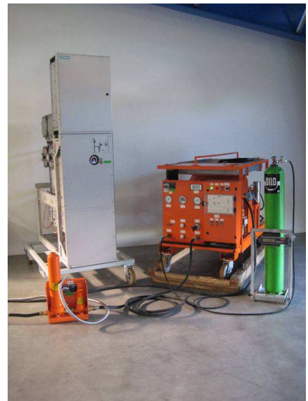
Figure 10: SF 6 gas re-use at manufacturer site
