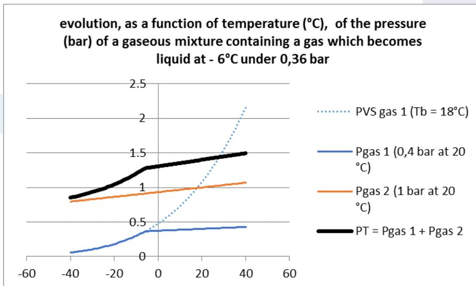
Figure 2: Evolution, as a function of temperature, of the partial pressure of 2 gases and the gas mixture comprising these 2 gases, where gas 1 ( $T_b = 18 \text{ °C}$ ) liquefies at  $-6 \text{ °C}$  at 0.36 bar
